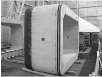
写真-3 推進函体 (1,800×2,800, L=1.25m)
